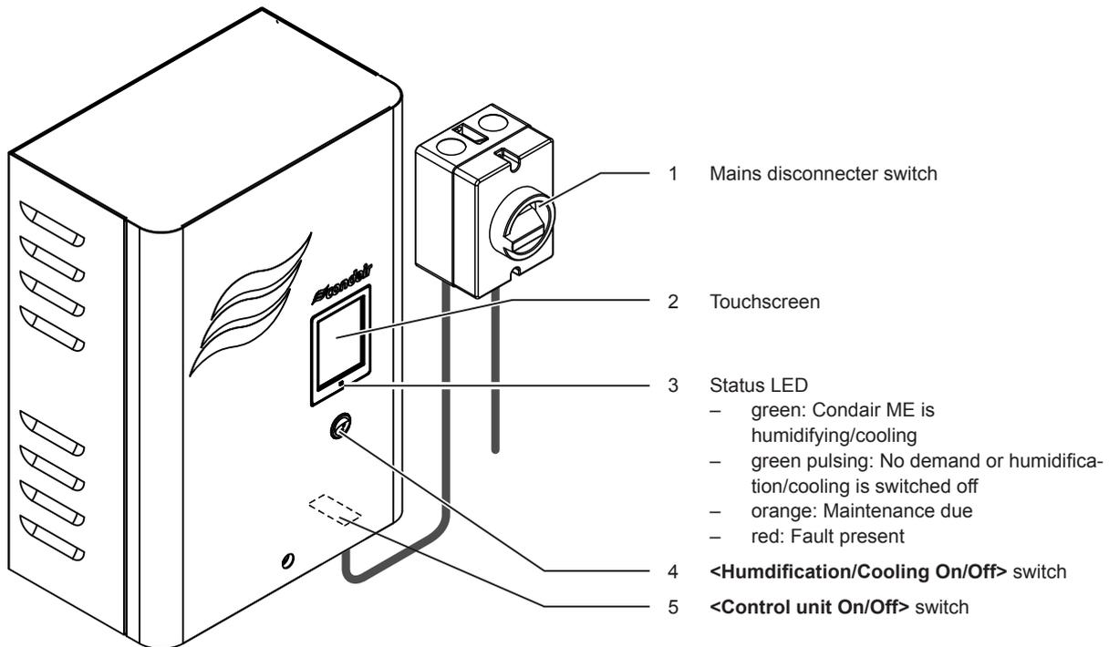
Fig. 10: Display and operating elements Condair ME control unit
