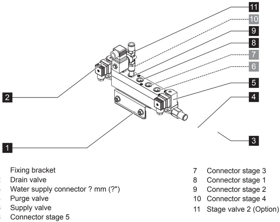
Fig. 3: Hydraulic module direct feed systems (figure shows layout for 2-stage control - option)
