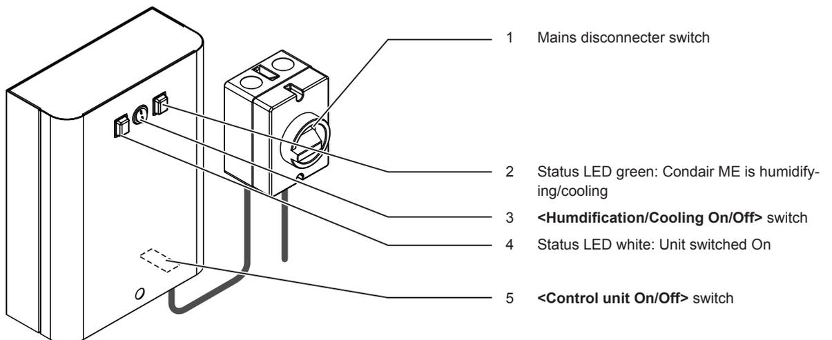
Fig. 11: Display and operating elements Condair RS control unit (Option)
