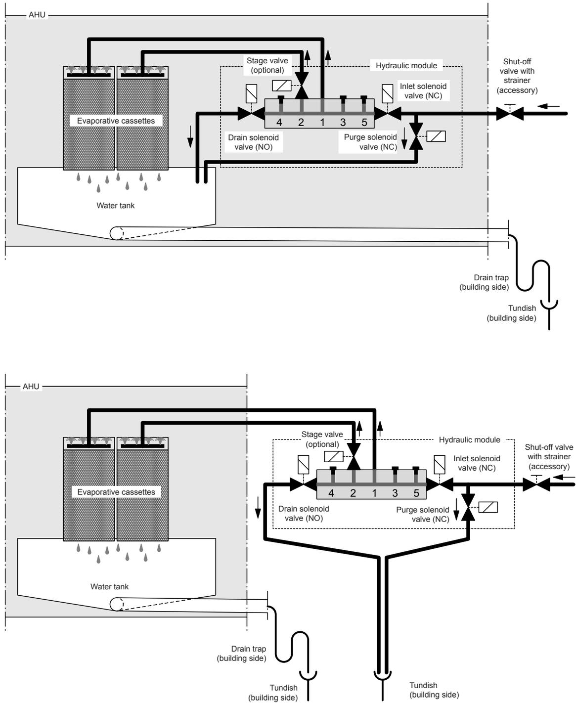
Fig. 9: Pricipal diagram Condair ME Circulating System (internally and externally mounted)
