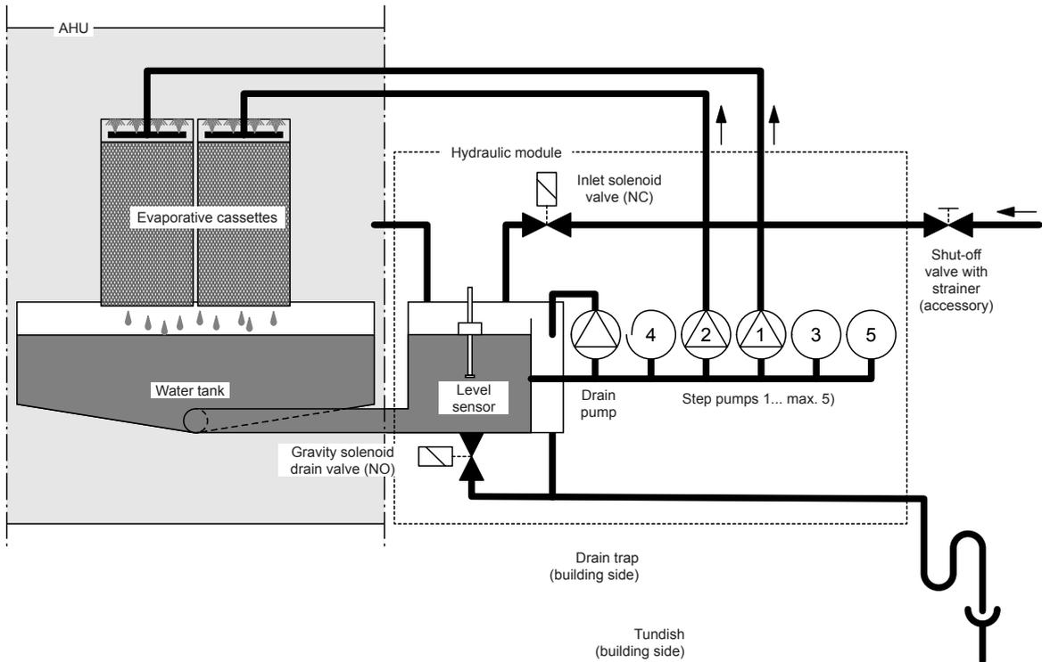
Fig. 6: Pricipal diagram Condair ME Circulating System (internally and externally mounted)
